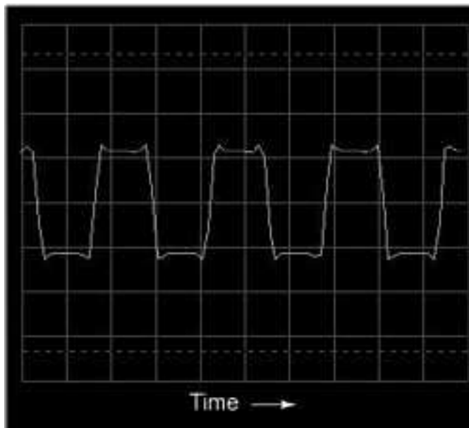
Figure 7.31: Oscilloscope time-domain display of a square wave
