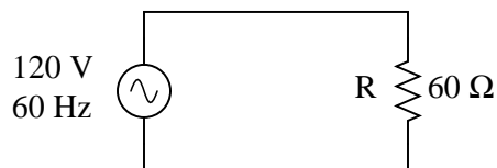
Figure 11.1: Ac source drives a purely resistive load.
